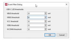
In Event Filter Dialog the user can set the noise threshold values. Only measurement exceeding the corresponding threshold will be logged.
