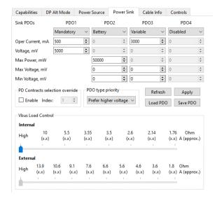
PDO Type: Definition of power source type (Disabled, Fixed, Variable or Battery)
