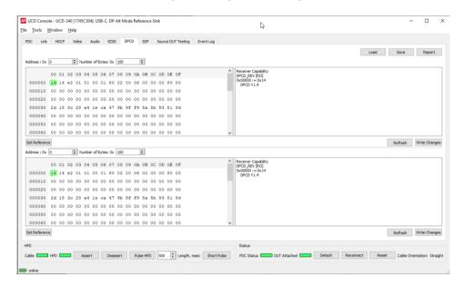
The *DPCD Decoder* panels on the right show the interpretation of the DPCD byte selected on the monitoring windows. The selected byte is shown with a green background.
