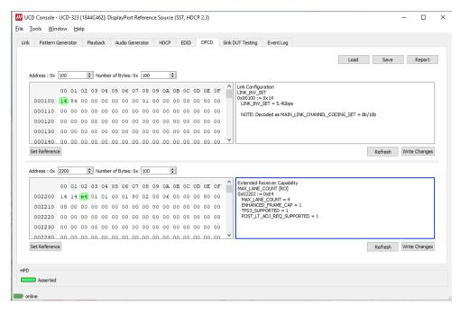
The *DPCD Decoder* panels on the right show the interpretation of the DPCD byte selected on the monitoring windows. The selected byte is shown with a green background.
