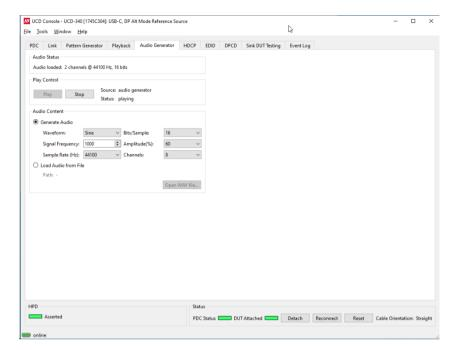
To load internally generated audio, select **Generate audio**, and adjust the controls to the desired audio format.
