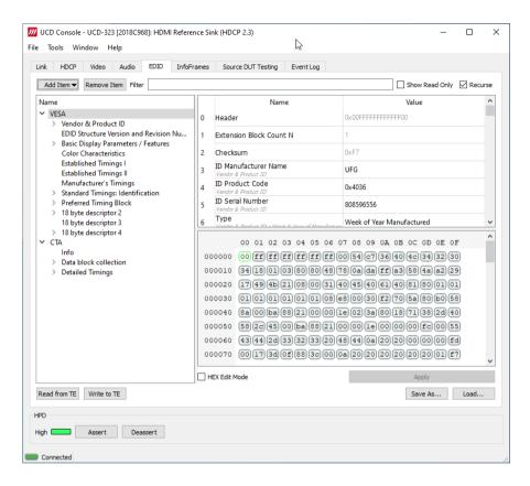
The *EDID Editor* main window is divided into three logical areas. The bottom part additionally contains the command buttons. The top-left portion shows the currently edited E-EDID blocks in a tree-form, and the top-right portion shows an edit control for the currently selected item, possibly a list of sub-keys and their names (The list is not shown for all values) and the HEX-view of the block collection.
