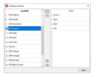
The order of Active items can be changed by selecting an item and moving its position in the list with up ▲ and down ▼ arrows.
