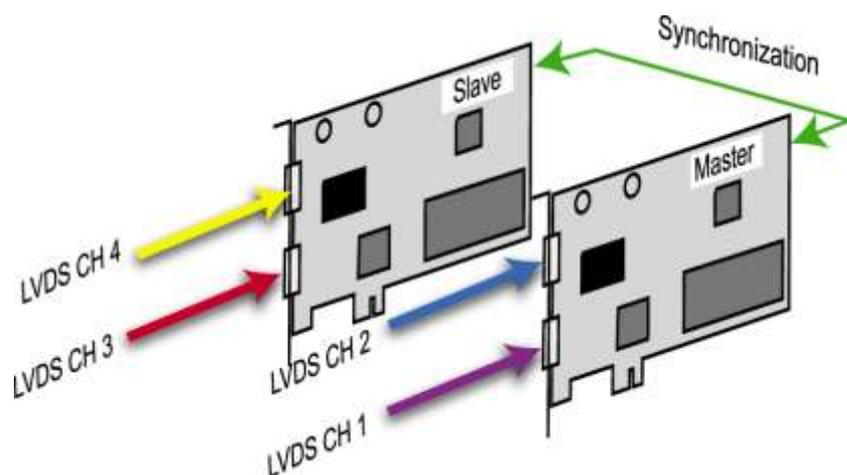
The mapping of the pixel data into LVDS data varies from one data source to another. In order to provide flexibility for the user UFG-04 LVDS features an internal data matrix for multiplexing the LVDS data to the input color bits. The multiplexer enables any pixel data combination to be used. It also enables the use of selectable pixel color depths. The setting of the multiplexer is identical for both input channels.
