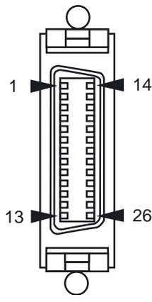
Pin-out of LVDS Input Connector CH 2 in UFG-04 LVDS
