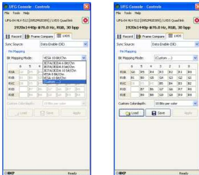
By selecting the **(Custom ...)** you can define a custom mapping in the matrix. Please note that the mapping of DE, VS and HS to bits 4 to 6 in lane C (RXC) cannot be changed. *Custom Color depth* field allows you to select between 6, 8 or 10 bit depth of color components.
