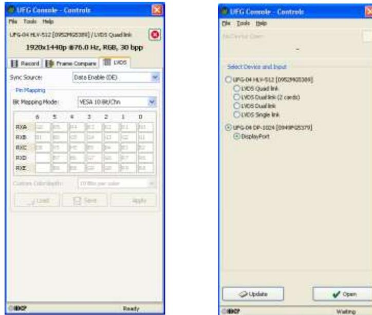
The *LVDS Acquisition Mode* is selected when opening the board. You can select between *Single link* and *Dual link* mode with a single board, and between *Single link*, *Dual link* and *Quad link* mode with two boards. The special *Dual link (2 boards)* mode uses Dual link mode to speed up the transfer of the captured frames to the PC.
