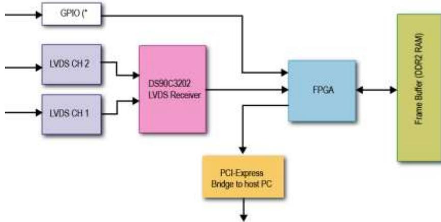
(\* GPIO (General purpose I/O lines) is used for synchronizing the master and the slave boards in a multi-board capturing configuration.
