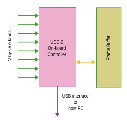
The image on the left shows the data flow inside the UCD-2 Vx1 device.
