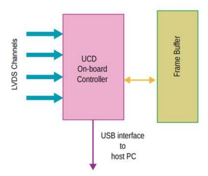
The image on the left shows the data flow inside the UCD-1 LV device.
