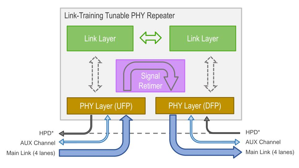
\*) LTTPR can either control or only snoop the HPD signal
