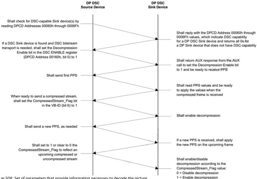
PPS = Picture Parameter Set. Sent as SDP. Set of parameters that provide information necessary to decode the picture
