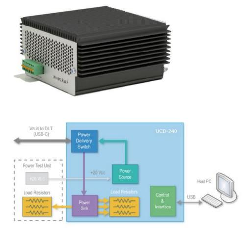
Unigraf *External USB-C Power Test Unit* enables testing extended USB power options. Please find below a matrix describing Power Source and Power Sink options of UCD-240 internally and with attached *Unigraf External Power Test Unit*. Please find description of controlling the power options with UCD Console later in this manual.
