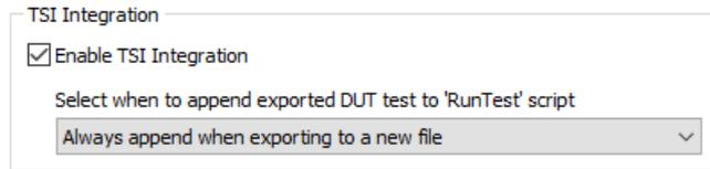
*Enable TSI Integration:* When selected, TSI Integration tool (*Tools > TSI Integration*) is enabled. When exporting test parameters in Sink / Source DUT Testing, test code is also appended for execution with TSI.
